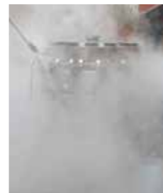
Under-going high pressure jetting test for IPX9k
